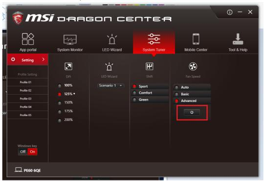
Default value setting would be like this picture. And depends on different model, the default RPM percentage would be different.
