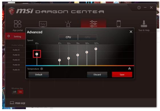
You can use the same way to setup GPU FAN RPM. Please click "Save" when you finish the setup.
