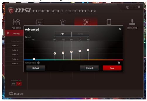
You can drag the percentage bar to fine tune FAN speed, drag up to increase FAN RPM; drag down to decrease FAN RPM.
